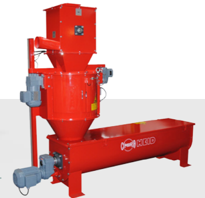
CONTINUOUS CHEMICAL TREATER For chemical treatment to protect kernels.
