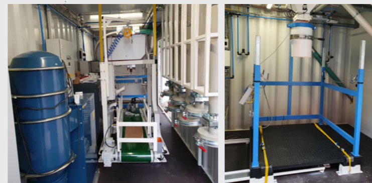
FILLING STATIONS Either in 10 - 50 kg bags or in big bags, or both.
