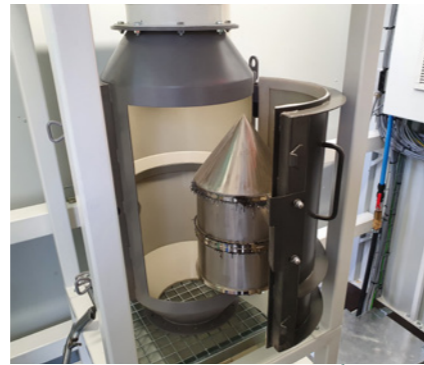
PIPE MAGNET To remove metallic parts.
