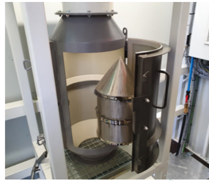
PIPE MAGNET To remove metallic parts.
