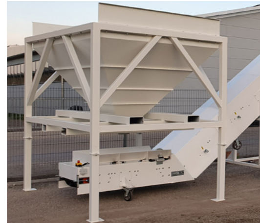
01/ Intake pit and belt conveyor
