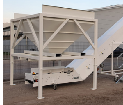
INTAKE PIT AND BELT CONVEYOR For simple and quick feeding of the processing line.
