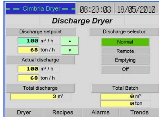
On the discharge control picture, the cubic meters treated and discharged are known from counting the strokes in the discharge system. From the typed in density of the grains the mass flow is calculated and displayed.
