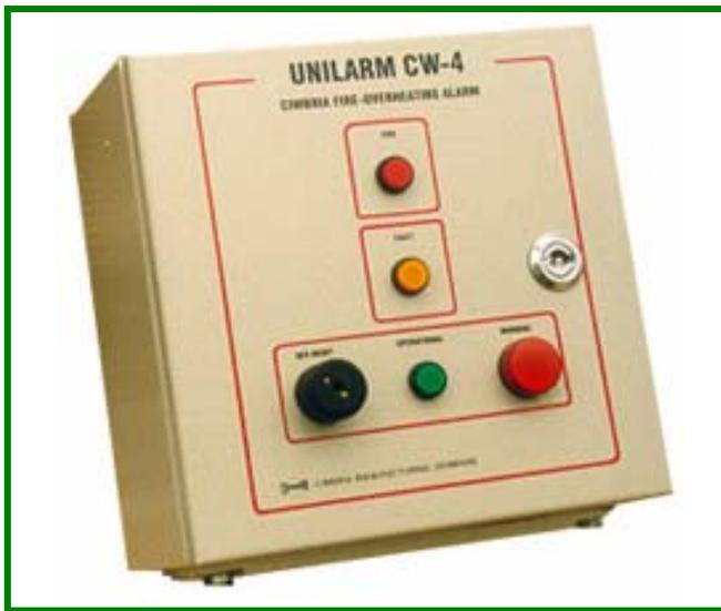
In case of alarm the fans and the heat source are automatically stopped and a red lamp at the control panel indicates alarm. The monitoring system is built into a metal box with indicators for operation, fault and alarm as well as a key reverser with on/off and reset functions.
